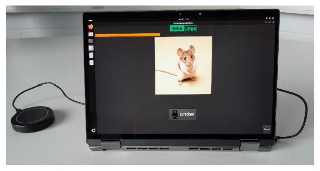
Figure 1: The hardware setup for the RehaLingo speech training
