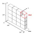
Figure 2: Patch-of-Interest (PoI): Data selection within DVS-OUTLAB
