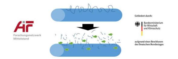
Figure: Schematic representation of the enzymatic degradation of a fiber Top: Polyester filament with a schematically continuous polymer chain (dark blue); Bottom: Polyester filament with polymer chain degraded by enzymes (green) into short and long fragments
