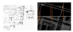
Figure 2: Left: Corner-based matching of building walls detected from a UAV point cloud (see Section 6) with CityGML model's walls. Right: Lines that are detected in the point cloud are matched with CityGML model lines.
