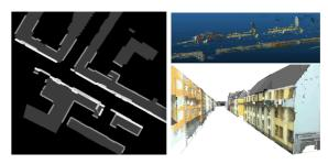
Figure 9: Knight street scenario: matching between line segments, thin point cloud, points projected to model walls
